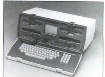
1981 Adam Osborne built the first portable computer, the Osborne 1. It cost $1,795 and weighed 24 pounds.
