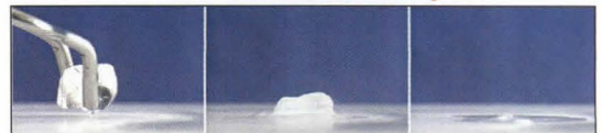
2002 Phase-changing materials, capable of storing more heat than water, begin to have application in wallboard and other materials that help buildings achieve energy efficiency.
