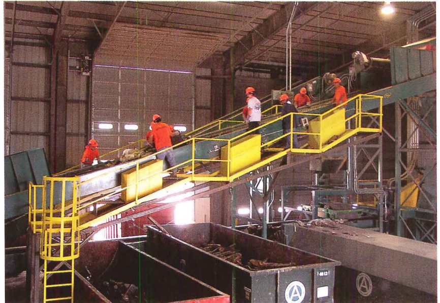
At the Phoenix C&D Recycling Facility in Des Moines, demolition waste is loaded on the screening deck and conveyor. Sorters inspect their picks and drop them into nearby bins.
