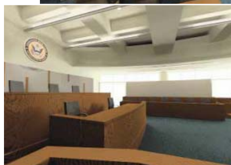
Arup tested the courtroom's acoustics (top) and helped build 3D models for lighting and sight-line analysis (above and left). The team noticed a potential glare problem behind the jury box (middle in image at left) during the CAVE walkthrough.
