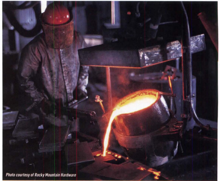
The bronze sand casting process.
