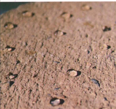
A concrete additive that repels water (page 159)
