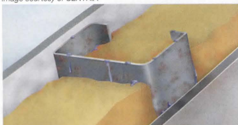
A steel stud wall assembly with insulation installed between the stud framing.
