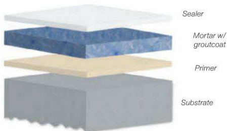
Configuration of decorative troweled mortar flooring.
