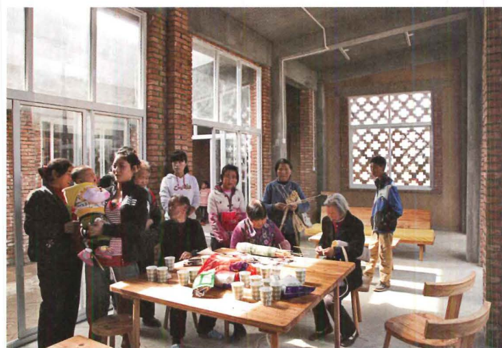
The architect was inspired to design the brick screen after a visit to the westernmost areas of China, including Kashgar in Xinjiang province. The screen helps keep the house cool in summer and warm in winter (above). An angled concrete roof collects and stores rainwater and provides a place to dry food (left and below left). Two women live in the house, which is also used for a women's weaving cooperative (below).
