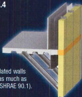
6" Traditional Stud Insulated Wall R-7.4
