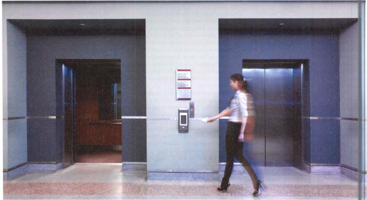
Elevator layouts traditionally are dictated by efficiency of core area and ADA rules, but destination-based systems remove this design constraint allowing more freedom in planning a lobby layout.
