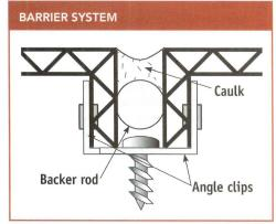
In a barrier system, caulk and backer rod form the seal between two composite metal panels.
