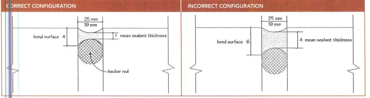
Left: The correct shape for caulk is hour glass with a ratio of bond surface to mean thickness of about 4:1.
