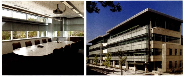
Left: Solar screen fabric helps to prevent glare and preserve views to the outdoors, while the automated shading system controls the position of the fabric on the window. Right: Siting and façade orientation each play a large role in determining what type of daylight is available at a window.
