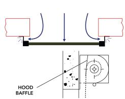
Rolling steel doors are useful in many buildings, but air leakage around the perimeter of the doors needs to be addressed to assure that they are energy efficient as well as functional.
