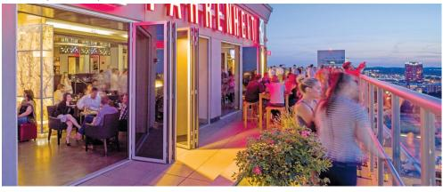
Operable glass walls can be used to provide complete flexibility of building design by allowing indoor and outdoor spaces to be combined when the walls are opened or sealed off and protected when closed.
