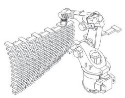
**BILLOWING BRICK** To convert an old industrial building in Shanghai into artists' studios and a gallery, architects from Archi-Union salvaged the bricks from the original structure. They created the new undulating facade (left and top) with the help of a bricklaying robot (above).
