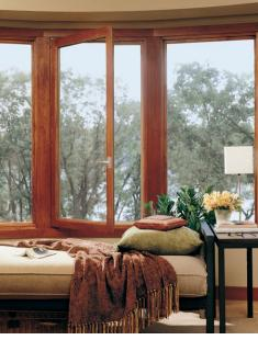
The type and function of operable windows can affect their energy performance, particularly in terms of air infiltration. The tilt-and-turn type shown here, which offers opening options, is generally the most energy-efficient type available from some manufacturers.
