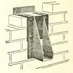
No. 4-Steel joist hanger for brick walls.
