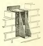
No. 4-Steel joist hanger for brick walls.
