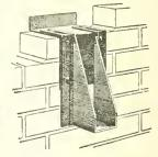
No. 4-Steel joist hanger for brick walls.
