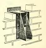
No. 4-Steel joist hanger for brick walls.
