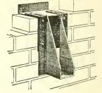
No. 4-Steel joist hanger for brick walls.
