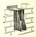
No. 4-Steel joist hanger for brick walls.
