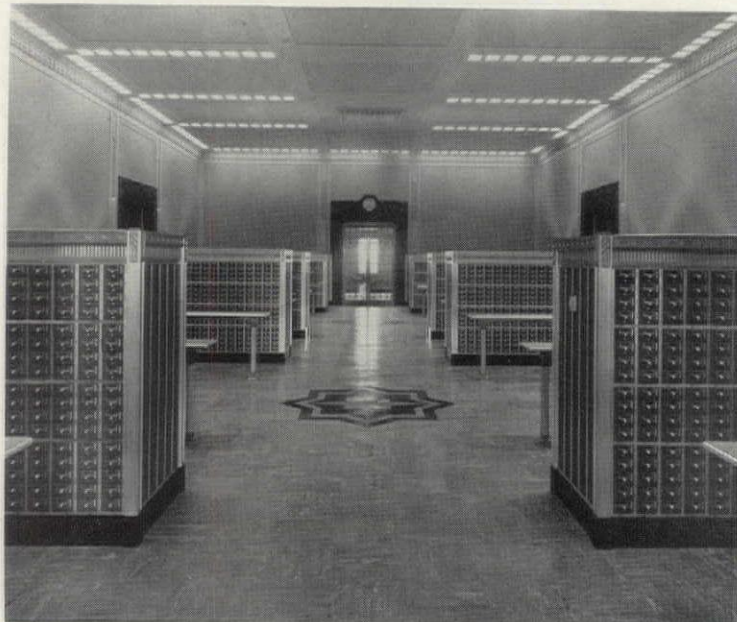
Card index cases with Formica morocco surfaced plates used as drawer fronts and as panels on the ends of the cases.
