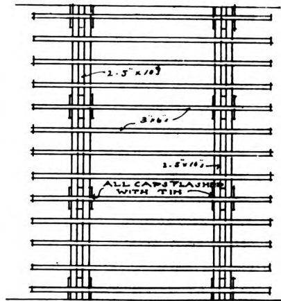
Plan of Trellis Work over Columns
