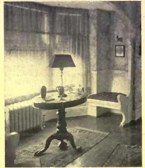
A special radiator enamel is now obtainable so that the iron can be made to match the color of woodwork or wall covering
