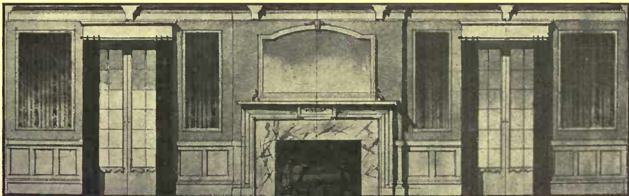
A side elevation of the room, showing the fireplace and the French doors to the piazza. Above the white wainscoting, the background paper is a putty color, the panels being filled with a striped and foliated fabric, held in place by a flat molding strip
