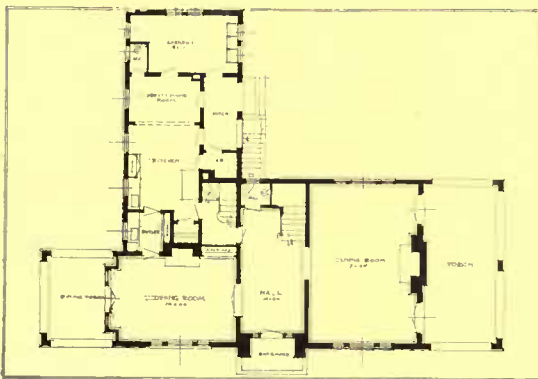
The house is rather larger than might be expected from the photograph of the front. A deep wing back of the dining-room provides more than the usual amount of space for kitchen, servants' dining-room, alcove, laundry and closet space. The smaller end porch is convenient for dining outdoors
