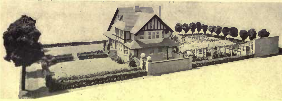
Windows are made of celluloid sheets, upon which white ink lines represent the divisions between the panes
