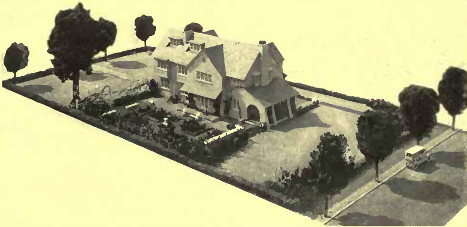
In order to prevent warping, it is better to use a base made up of cardboard layers glued together, rather than a single board
