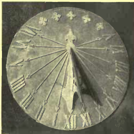
The completed dial worked in brass as it appears with the gnomon and hour lines in position
