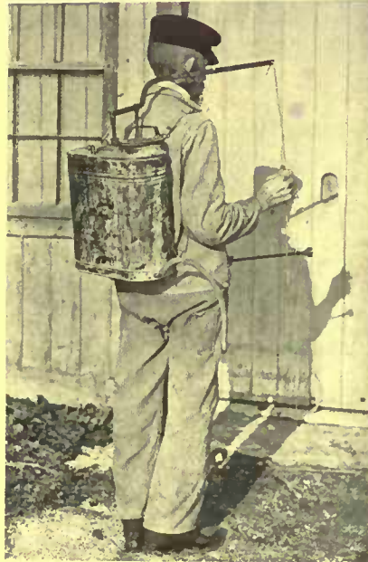
The knap-sack sprayer is worked by a lever that runs over the shoulder
