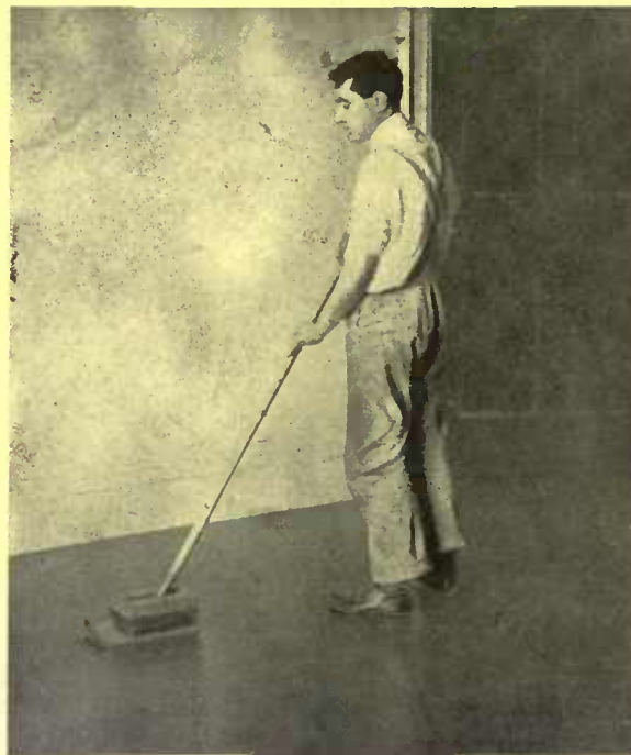
With a weighted floor brush the labor of keeping the hard wood in condition is materially lessened
