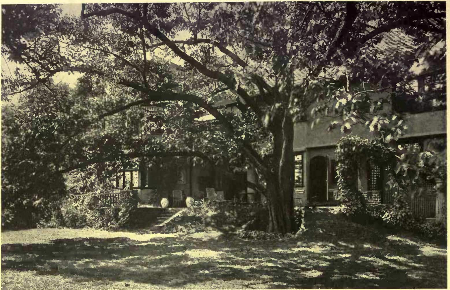
The great oak tree determined the physical form of the house and became a factor in shaping its plan. In summer it shades the entire side of the house and the brick-paved terrace. In winter, when the leaves have fallen, the tree keeps off no desirable sunlight
