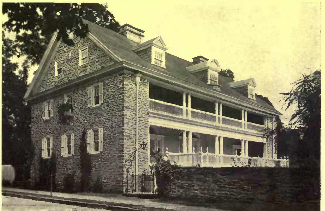
The loggia type of porch may sometimes be used as in this interesting two-tiered example where the porches run the length of the house
