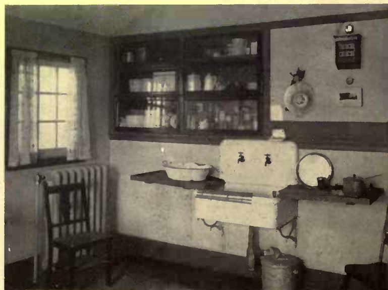
In this small country house kitchen the cupboard doors lift up and slide back like those of a sectional bookcase
