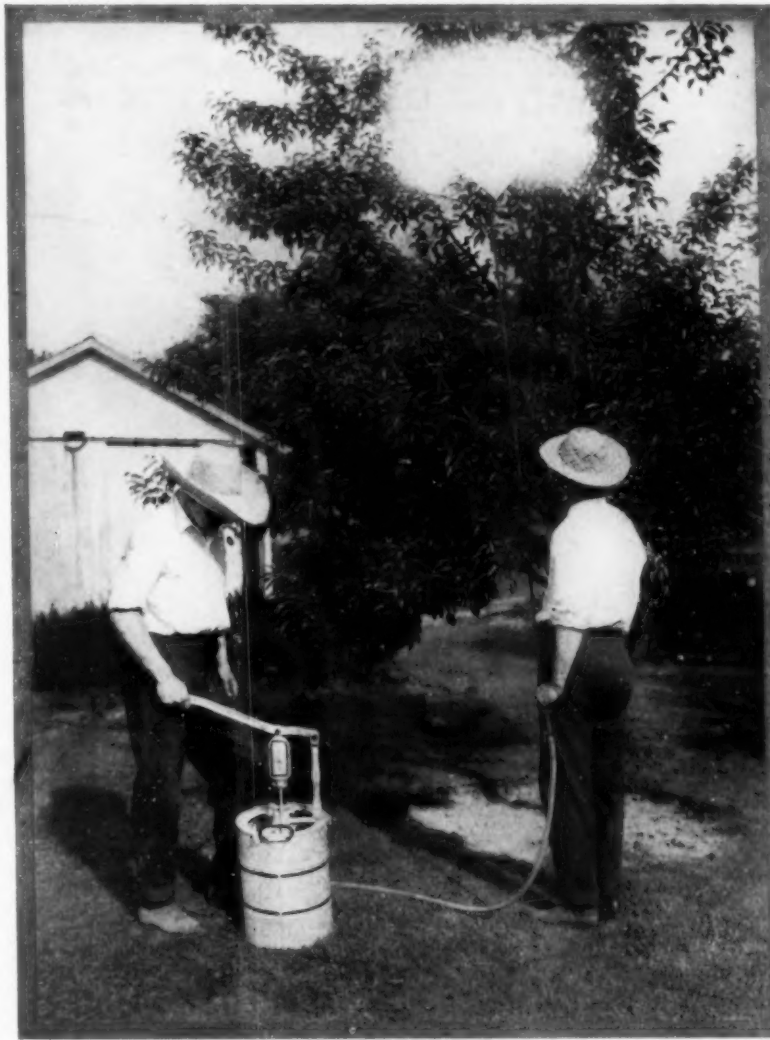
For the small orchard of dwarf fruit trees a portable machine handled by two men will be sufficient. Here again the extension nozzle is necessary
