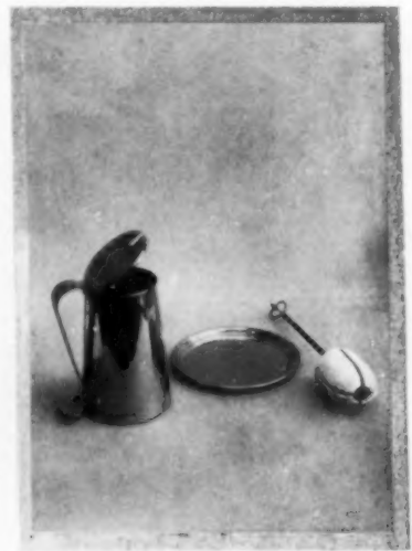
A product of "safety first"—a fire starter, with a stone torch to soak in oil
