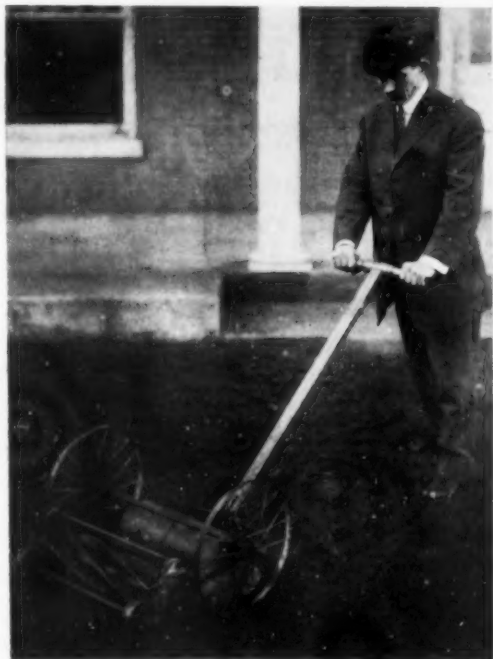
A roller mower, with demountable cutter and steel-carrying wheels, adaptable to the small place
