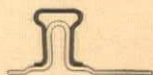
Most strips have the rib (white line) but only Higgin Weatherstrips have the patented Insert (black line) that really keeps the weather out.
