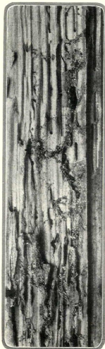
A section of flooring from a house in Iowa showing the action by subterranean termites on wood which is in close proximity to the ground
