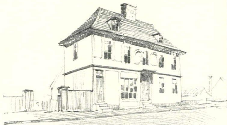
Character is given to the house by the steep roof pitch and the wide overhang of the eaves. The wide courses give horizontal emphasis to the design
