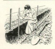
Dig the trench 2' deep. To assure accurate depth measure down 4' from line you have strung after marking grade. Dig as narrow as possible. Don't dig so deeply that you'll have to fill in again as tiles must set on firm base.
