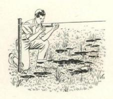
Put a stake at low spot of wet area to be drained. Tie twine to stake 2' above ground. Run string out 50' to 100'. Attach line level and secure string at level position to second stake. Figure slope by measuring from string to ground.
