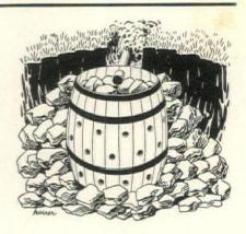
The outlet may be a stream, drain or a dry well. To make a dry well bore 1" holes in a barrel. Set barrel in a pit on 1' bed of rock deep enough so tile opens into it. Fill and surround with broken stone. Cover with tar paper, fill in soil.
