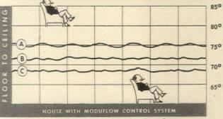
Temperature at ceiling. B—at five foot level. C—at floor, See how Moduflow smooths out the up-and-down temperatures caused by ordinary control systems. Without Moduflow, temperature varies as much as 20 degrees from floor to ceiling. With Moduflow there is comfort temperature from ceiling to floor.
