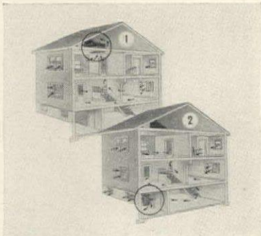
AIR CHANGER works something like paddle wheel to draw cool night air through house, expel it outside. Installation in either attic (1) or basement (2). Minimizes fan noise. $350 to $400 depending on construction of the house. Eagle Picher Co.
