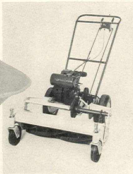
HEAVY-DUTY POWER MOWER for large grounds, 24-inch cutting width. Pincor, $225 f.o.b. factory. Pump, plow, sickle, roller are extra attachments made for it.
