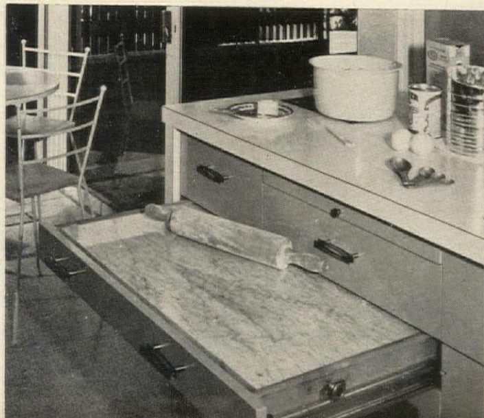
▼ Pull-out marble slab on heavy metal gliders is space-saving asset for dedicated pastry cook.
