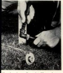
stic pipe is easily cut with a strong and special angles and connectors e placed and replaced as required.
