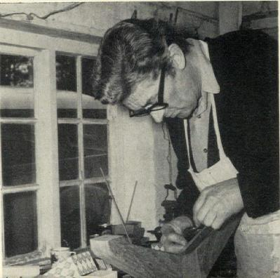
After being sawn, the timber is left to season for at least a couple of years and frequently kiln-dried after seasoning. By careful selection and care, the craftsman's timbernightmare of twisting is avoided. The natural characteristics of the timber are cosseted and exploited: a log with a gentle curve will serve well enough for a chair leg, necessitating the minimum of cutting across the grain.
