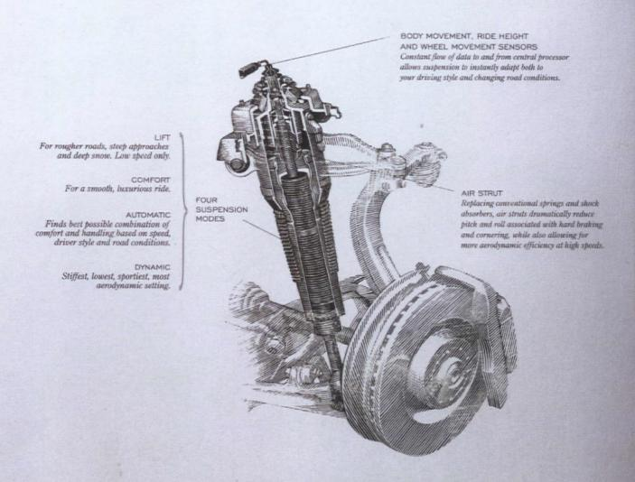
Fig. 21. - Adaptive Air Suspension, lets you alter the ride of the A8 L to individual driving styles and road conditions.
