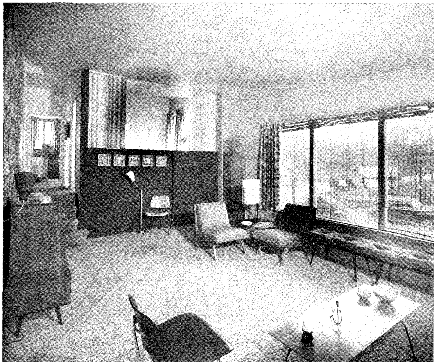
Continuity of space ties living area to multipurpose room at higher level. Coat closet near entry is same height as bookshelves facing into higher-level room. Living room has more glass area than most merchant-built splits. Louvered windows are stationary; panels behind them are movable for venting.
