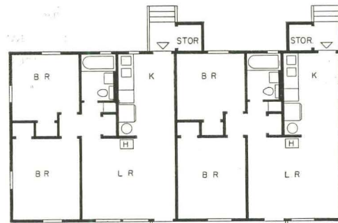
PHMI 'DEMOUNTABLE' two-bedroom duplex is built of insulated plywood panels with flush exterior joints, rests on masonry piers. It comes with space heater, electric stove, refrigerator, water heater, softwood floors.
