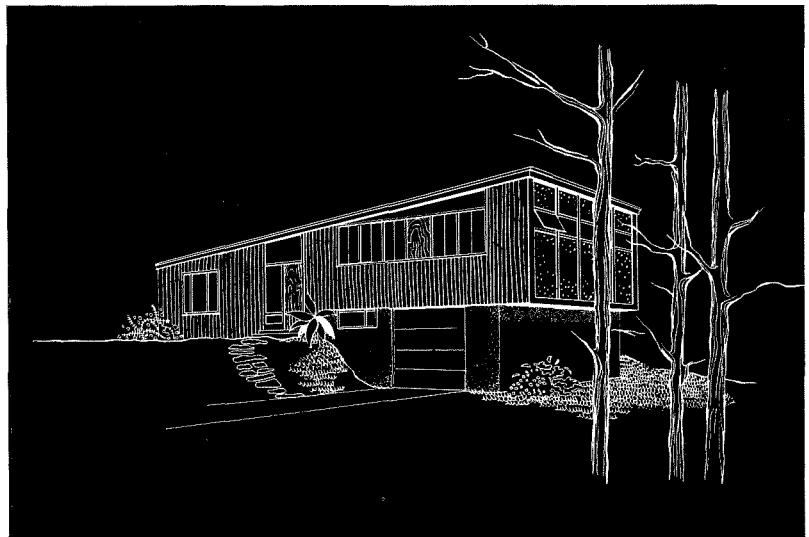
Sales success of earlier Grossi model (below) prompted Builder Kruvant to try more advanced design (above). Shed roof eliminates roof break, flashing, complicated carpentry. Model shown is best where lot affords privacy at one end or is at end of street. Alternate design has windows in front.
