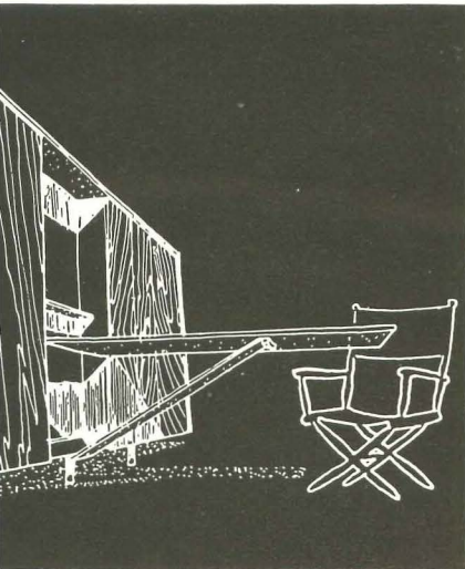
Built-in outdoor table folds down out of storage bin. When folded up, it serves as a bar. By Warren W. Weaver.
