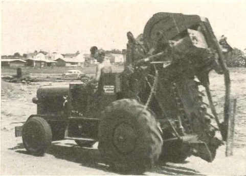
Mobile trencher can easily make 90° turn (above), speeds off to next foundation job when finished.
