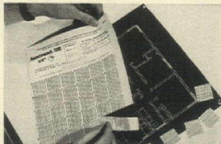
DESIGN AND LAYOUT is simplified by Anaconda's free layout kit of printed, gummed PG scale drawings, which show precise layout of heating panels on blueprints.
