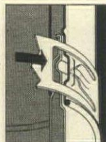
UNLOCKED TONGUE RELEASED — PIPES EASILY COUPLED AND UNCOUPLED
