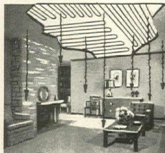
Cut-away view of Sunwarm installation shows how clean, uniform heat flows from concealed cables.
