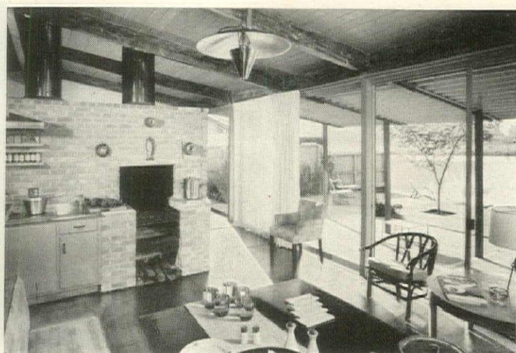
Massive brick wall divides family room-kitchen and living room, has barbecue, built-in stove, decorative copper flues.
