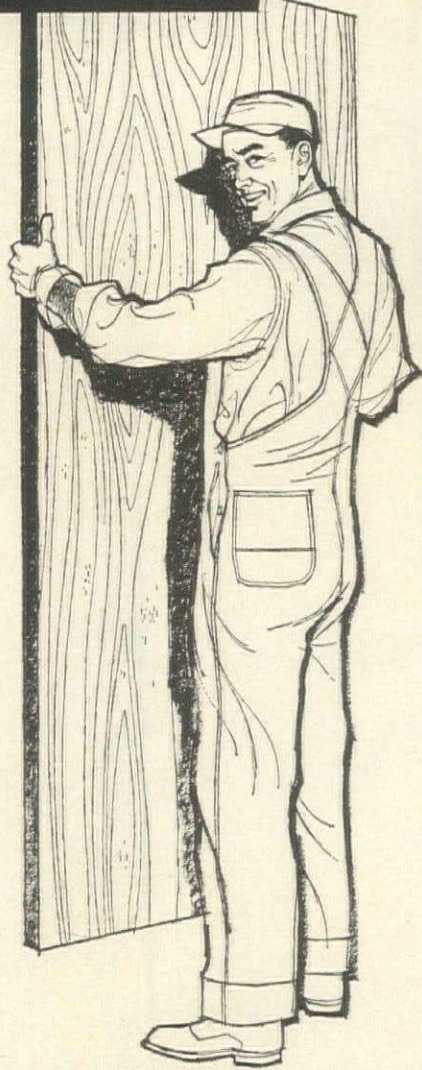
A standard 2-6 x 6-8 door weighs only 30 lbs. It's easy for one man to install a REZO door.
