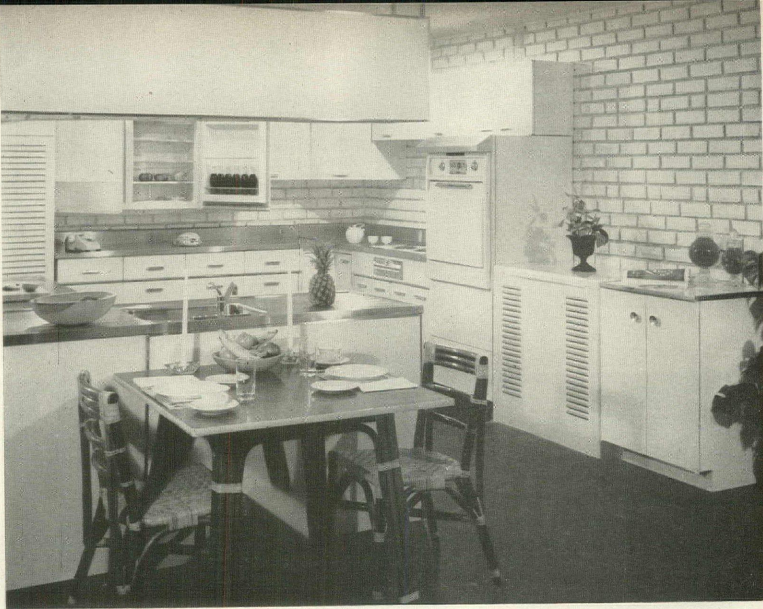
Package kitchens , like this one in $26,900 model, offset any buyer's doubts about lack of cellars, Jalonack says. Heating unit, right center with louvered front is in kitchen of three models, serves as counter-top, eliminates utility room.
