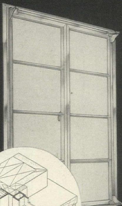
INTEGRAL FIN-TRIM CASEMENT . . . A Ceco feature window in aluminum. Outside fin and trim are extruded as an integral part of the frame member. Fastest installation ever for frame, stucco, brick or masonry. Place in rough opening, nail in place, bring up siding and caulk.
