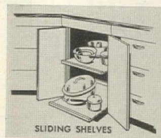
FITTED UTILITY CABINET
