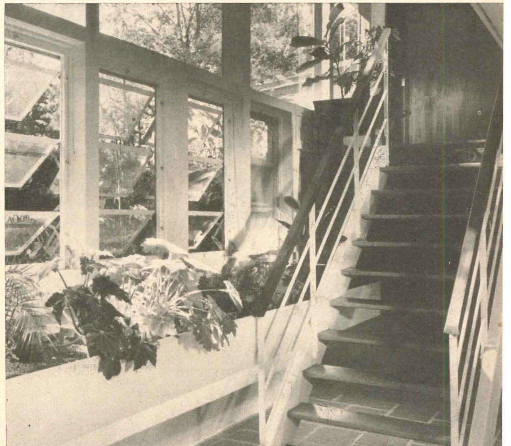
Trim stairs lead up to entrance. Balusters are metal, handrails and treads are oak.
