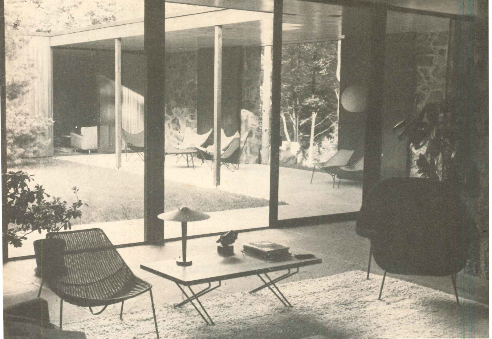
Living area faces patio on one side, Connecticut woods on the other. Downlights in roof overhangs reduce reflections in glass at night.
