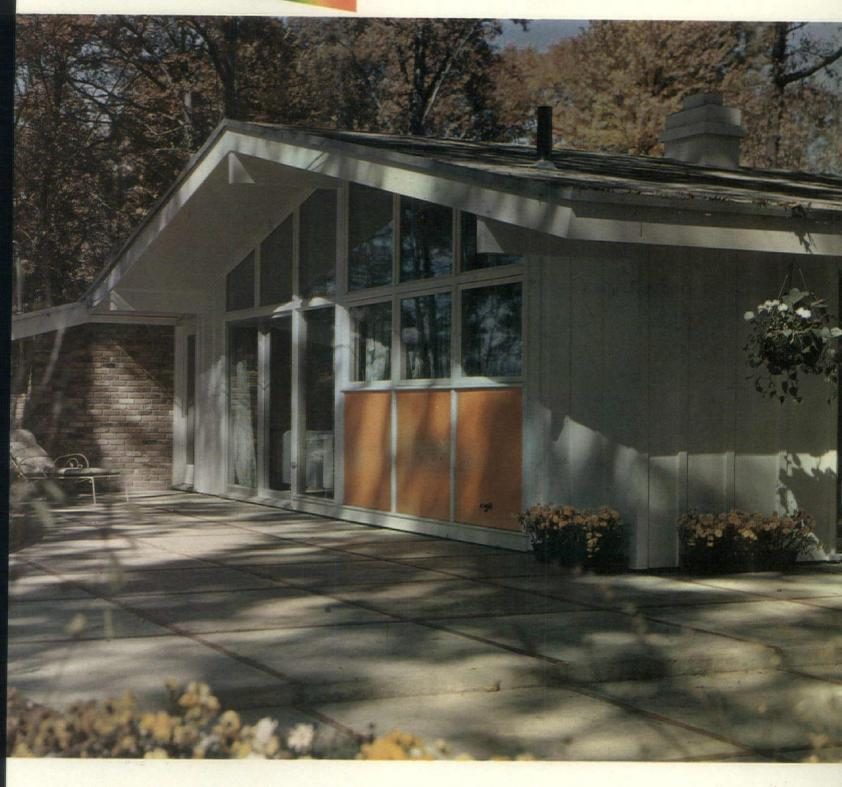
The exterior finish walls are built with pre-primed Johns-Manville Asbestos Flexboard which lends itself beautifully to the authentic board and batten styling of the true California ranch style architecture of the Mark 58. This siding material is rotproof, fireproof and weatherproof. In addition it provides an excellent paint base, not subject to the wide variation in paint holding characteristics of other siding materials.
