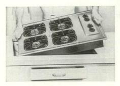
**Gas drop-in top** doesn't need a front cut-out and it is only 3" thick, so it will fit above the drawer space in most base cabinets. Modern Maid unit can be simply installed in tile tops, too, for a custom look; and once in place, it pulls down flush to cabinet—so there's no way for spillovers to run into cabinet.
