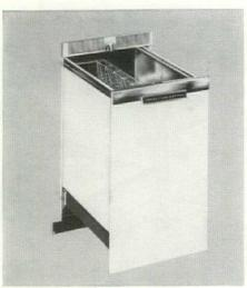
**Small dishwasher** uses only about 6 gallons of water, maker says, but by recirculating water under pressure at the rate of approximately 80 gallons per minute, it provides the equivalent of 500 gallons. The unit is top loading and is said to hold as much as larger dishwashers. It is 18'' wide,  $31\frac{14''}{14}$  high to allow for  $1\frac{1}{2}''$  countertop and  $\frac{1}{4}''$  adjustment to floor. Depth closed is 24''.
