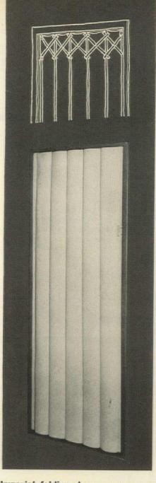
**Imperial folding door** uses two vertical synchronized pantographs, one at top of door, other near the bottom. Synchronized action of the two pantographs is achieved by connecting opposite pivot points with vertical steel rods and fastening the vinyl-plastic covering to the rods. Door covering is carried to within <sup>1</sup>/<sub>4</sub>" of top of frame to conceal track and eliminate need for cornice or valance.
