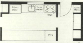
Floor plan shows the efficient location of the Westinghouse Space-Mates Laundry Twins at the end of utility hallway. Adjacent wall space is used for built-in storage and linen closets. Oven is located across aisle from built-in range platform.
