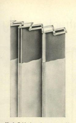
**Magic-Fold door** has pantographic action to keep folds uniformly spaced, requires minimum stacking space (only 41/4" for 32" opening). Door is made in 41/4" panels so it can be set into a standard-width door jamb. Full-length Masonite baffle cores in the heat-sealed vinyl pockets keep the door rigid regardless of heat and humidity and help insulate against noise. You can get a variety of handles and locking devices, and even matching top trim that looks like a valance.
