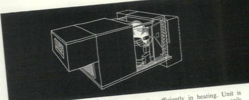
Packaged heat pump is air-to-air exchange system with electrical resistance coils at left end for supplemental heat when temperature gets too far below freezing for the heat pump cycle to function efficiently in heating. Unit is usually installed with condenser coils
