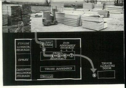
Production flow (diagram keyed to photos by numbers) begins when uncut lumber is fork-trucked from outside storage stacks (above) to saws in shop. Once work reaches panel assembly line (4), it rides through shop on roller conveyors.
