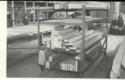
Cut-to-size lumber is stacked on this four-shelf hand truck, which is pushed to assembly jig by handler. Truck was designed by shop superintendent—holds enough material for a half-day's work. Frame is welded steel; shelves 3/4" plywood.
