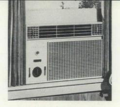
**Room air conditioners** are offered in capacities of 1, 1½ and 2 hp. Five of the 11 models in the line have reverse cycles so they work as heat pumps. Features of the new line include dehumidification control, electrostatic filters and flush mounting with interior wall. Slide-out chassis eases installation and service.
