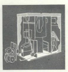
**Compact new furnace** (48" high, 25" wide, 53<sup>1</sup>/<sub>2</sub>" long) has a rated input of 119,000. All controls are mounted in front for easy servicing. A heavily baffled radiator lengthens fire travel.
