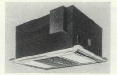
**Fan-light-heater** combines a squirrelgage exhaust blower, two 60-watt lamps, and a 1,450-watt radiator-convector. Automatic damper prevents back drafts, blower recirculates warmed room air when heater is on.
