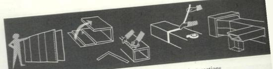
Prefabricated duct system of glass fiber board covered with aluminum foil is shipped in flat sheets, prescored for easy forming. Strip at edge of panel is removed to leave aluminum foil edge for stapler. Special tape goes over stapled flange and is used to cover butt joints of end-glued duct sections. Special sections (for corners, decreas-
