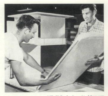
WESTINGHOUSE REFRIGERATOR, 1957: Walls of unit consist of foam-core sandwich with two metal skins. By scoring sandwich along definite lines, units of any size may be formed by simple folding process.
