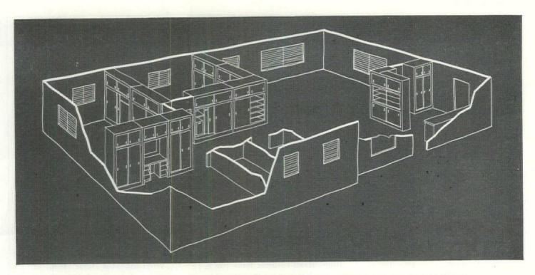
CUTAWAY PLAN shows how you can divide interior space with storage units. From stock pieces you can assemble units (below).
