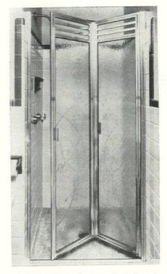
**Folding glass shower door** is primarily designed for small bathrooms where space does not permit a swing door. This new Permalume model folds into the shower stall so it doesn't protrude into the room. It comes in widths up to 36", has a standard height of 66" above the curb; with grill, it is 72" above curb.
