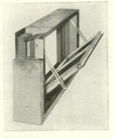
**These basement windows** eliminate need for metal bucks, wood forms and lintels with brick veneer or frame. They are 8", 9", 10" deep—full thickness of walls.
