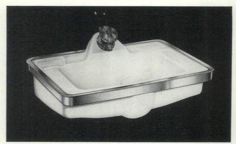
**New counter-top lavatory** features a new fitting called Uni-Dial, which allows user to control temperature and flow of water with one hand. Dial is tilted back and forth to control flow, turned to left or right for desired temperature. Water volume can be changed without affecting temperature, and vice versa.
