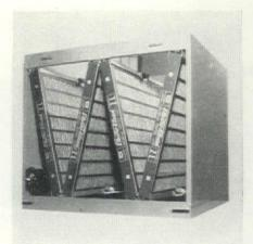
**Electro-Klean filter** eliminates dust, dirt and airborne pollen in the average house and uses less current than a 10watt bulb. The electronic filter is installed in the return air duct of heating or air-conditioning system, traps dirt in an electrostatic field with over 84 sq. ft. of filtering surface.
