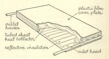
NEW FLAT PLATE COLLECTOR for solar heating. Details in text above.
