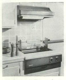
"Electramic" broiler contains two special heating elements above a bed of ceramic coals. The ceramic is removable and can be washed. You can install this charcoal-less barbecue in kitchen, family room or on a patio. The broiler mounts on any cabinet 24" square and 28" high. That will place the hardwood cutting board top (which fits over the unit) about 1¼" above a 36" counter top. Installation should be made to include a ventilating hood, company says. Stanthony Corp., Los Angeles.
