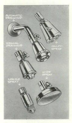
Five new showerheads have one thing in common—a heavy phosphor bronze spring which keeps a constant self-adjusting pressure between ball joint and packing. Self-draining and manualdraining units have corrosion, limeand wear-resistant nylon faces. Multispray is variable from fine needle to flushing flood.
