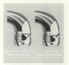
**Water-saving aerator** is said to save about five gallons of water per minute by a new design which mixes a little water with a lot of air. Mel-O-Flo Jet Aerator has a gear plug plus a wide mesh screen. When faucet is turned on, water pressure pushes gear plug down and water is aerated. When the faucet is off, spring raises gear plug so particles can be flushed out.
