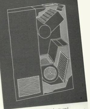
Heat-pump air conditioner heats and cools with gas firing. It measures 26"x62"x79", has heating capacity of 120,000 btu per hr. input and cooling capacity of 60,000 btu per hr. Cooling and heating coil is at upper right; air intake filter, lower right. Only moving part in the unit is the blower. Arkla-Servel, Evansville, Ind.
