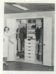
**Bi-Fold door unit** operates without guides, tracks or pivots. Doors are hung on regular full-mortise hinges and a spring in mortise at top of door passes over hinge pin to give automatic folding and unfolding operation. Spring holds doors straight when closed, keeps them folded when open. Two-door unit for openings up to 3'; four-door units for openings from 3'-6'. With split jamb, installation takes about 20 minutes. Ready Hung Door, Fort Worth.
