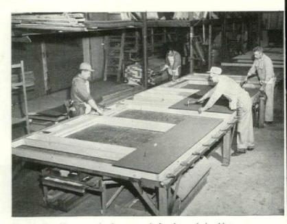
Big jig with pneumatic clamps speeds framing and sheathing of panel. Lumber is laid out with top and bottom plates aligned against clamping bars. Clamps, actuated by a single pushbutton, force plates against stud ends before nailing.
