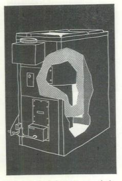
**New gas-fired furnace** uses singleport, up-shot burner for clean efficient fuel consumption. Five models have btu per hr. ratings at the bonnet that range from 64,000 to 152,000. Automatic humidifier is optional.
