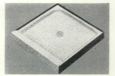
**All-terrazzo receptor** has its own built-in sill. The new Biltmore is made in one piece, doesn't need a lead or copper pan, and is claimed not to be affected by average building settlement. Shoulders are 1" high to keep shower walls well above area where water collects. Square models, 32" x 32" and 36" x 36", corner model, 36" x 36".
