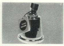
**Shower head** gives 60 streams of water which can be tuned to tingling, gentle or foamy washing action. Live rubber diaphragm in shower head is pierced with 60 slits. Water enters main body of shower head which is a large mixing chamber for incoming water to reach uniform temperature. Metal plate gives it a further swirling action.
