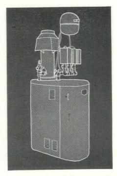
**Complete package boiler** comes with air pressure tank for closed system, top, and zone control package, middle right, with relay, transformer, high-head pump, pressure reducing valve and air vent. 100,000 to 200,000 btu per hr. Edwards Engr., Pompton Plains, N.J.
