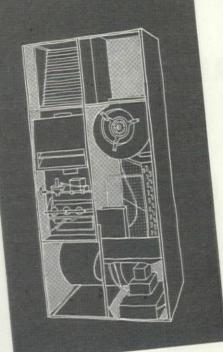
Heating-cooling air conditioner is packed into a unit 343/4" wide, 28" deep and 72" high. Heating capacity is rated at 100,000 btu per hr. input and cooling capacity at 23,200 btu per hr. Condensing coil is at right in picture and evaporator at top left above
