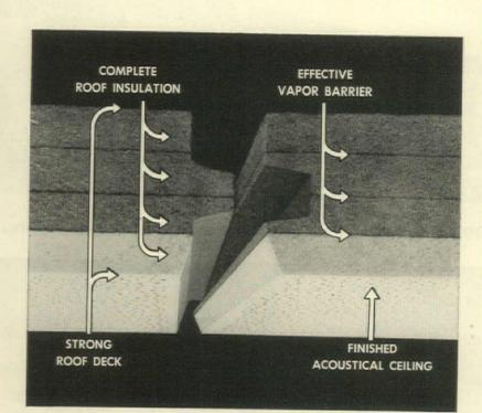
New Armstrong Cushiontone Roof Deck is a 4-in-1 material that provides roof deck, complete insulation, multiple vapor barriers, and finished acoustical ceiling in one fast, simple application. It needs only beams to support it and built-up roofing to weatherproof it.
