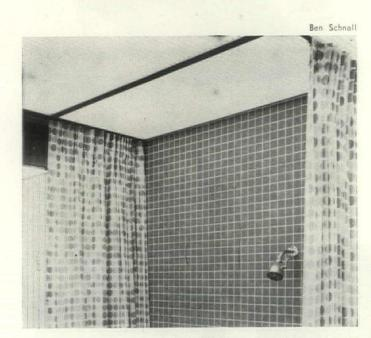
LUMINOUS BATHROOM CEILING, 1957: Fluorescent-and-plastic ceiling in this bathroom assures even, shadowless light, good for shaving, make-up. Designer: G. Luss.
