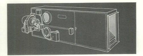
**Contour flame** of this furnace is made by down-sweep burner, heats all the primary surface of heat exchanger evenly in seconds. Models from 81,250 to 150,000 btu per hr. input are all only 57<sup>1</sup>/<sub>2</sub>" high. They occupy only 4.3 sq. ft. of floor, have AGA approval for zero clearance.
