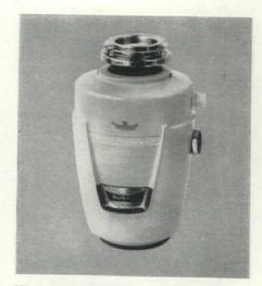
**King-size disposer** was designed to meet the needs of larger families. "Imperial Hush" is encased in a noisedeadening polystyrene shell lined with  $\frac{1}{2}$ " of fiber sponge. Its speed in disposing of waste is claimed to be 1.8 times as fast as any similar unit; and because of its size, long bones, corn husks and melon rinds can be fed in without first being broken into segments.
