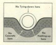
won't float-no need for anchoring. All your men do is position duct and pour concrete.
