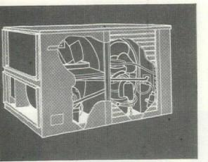
**Packaged air conditioner** has a cooling capacity up to 40,000 btu per hr. in the big 45"x35"x26" size. Smaller size, 20,000 btu per hr, measures 36"x26"x20". A vaporizer attached to condenser propeller blade uses evaporator condensate to increase condenser efficiency. The big unit contains a twin refrigerant system to provide two-stage air conditioning with better humidity control and more effective operation.
