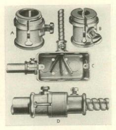
New connectors, one for joining conduit (A) and one for joining BX (B) to terminal boxes are a snap-in type attached without nuts. No wrench or pliers needed—connector snaps to box. Badger Die Casting Corp., Milwaukee.
