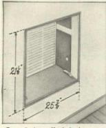
**Case is installed** during construction—mounts in any kind of wall. Panel protects opening until building is completed.
