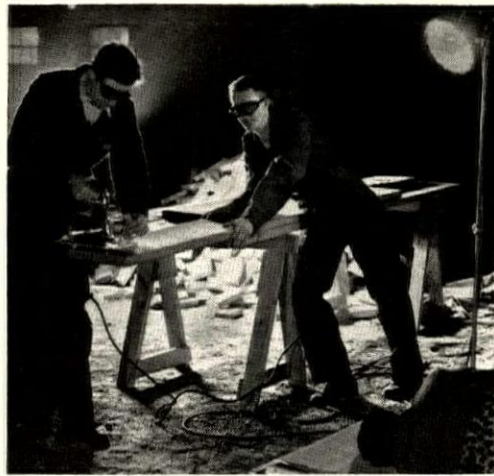
4:00 A.M.: It's 18 hours since the test began. Technicians will spell each other. The saw has used 10 blades and has cut over 4000 feet of lumber so far.
