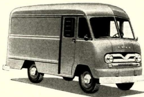
New Ford Parcel Delivery chassis. Four P-Series chassis with GVW's from 8,000 to 17,000 lb., for up to 525-cu. ft. custom bodies.
