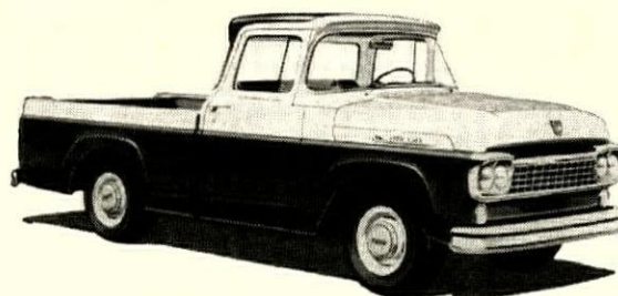
New Ford Styleside pickup. Modern Styleside body is as wide as the cab and standard at no extra cost . Conventional Flareside box available.
