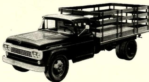
New Ford F-500. Rugged, versatile 1½-tonner with 15,000-lb. GVW. Two wheelbases for 7½- to 13-foot bodies.
