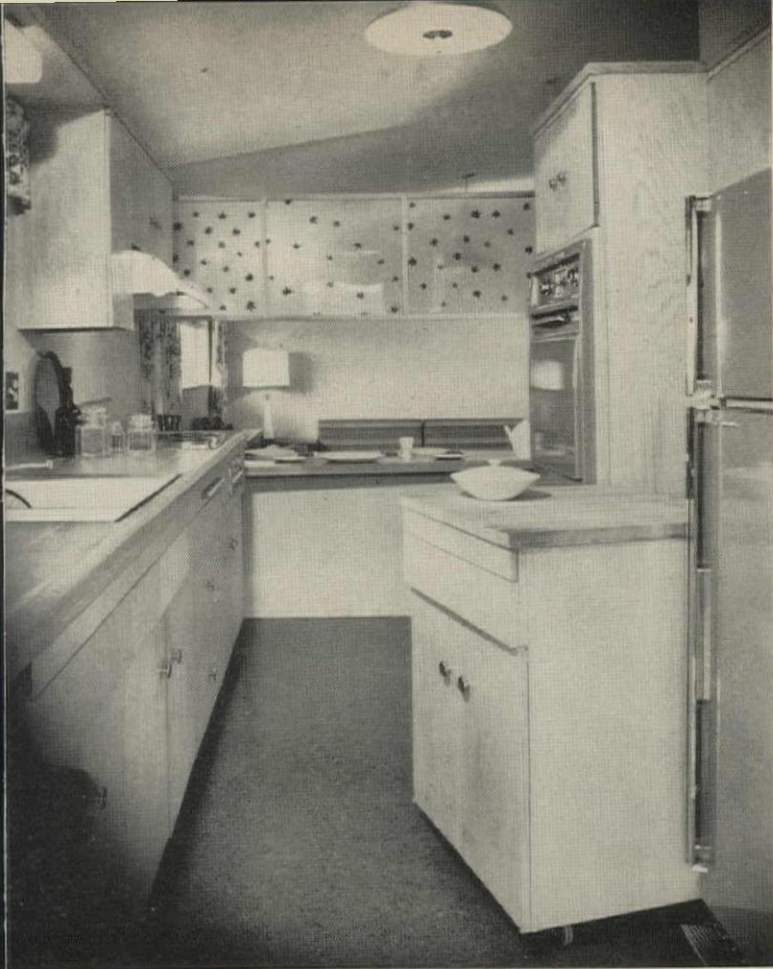
CABINET ON CASTERS is a self-storing unit that does double duty as a kitchen counter and cabinet and as a rollaway serving cart. Its top surface is a laminated hardwood chopping block.
