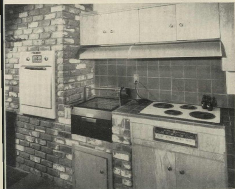
CHARCOAL BROILER with electric spit is a kitchen feature in College Park's fastest selling model. It's vented by the same hood as the range. Clever touch: charcoal storage compartment under the barbecue unit.
