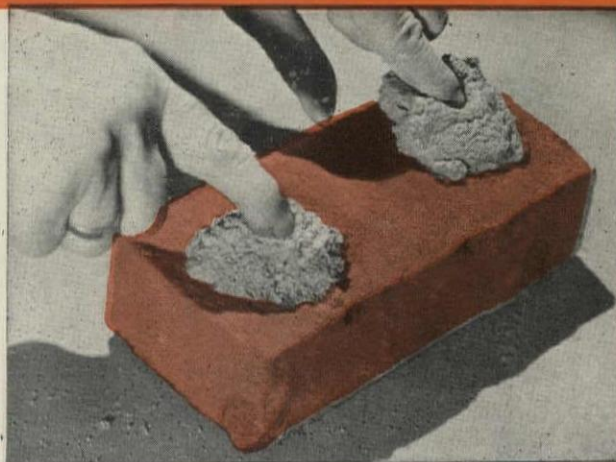
The one that stays plastic longer will be the one having the highest water-retention. Feel the difference with Brixment mortar!
