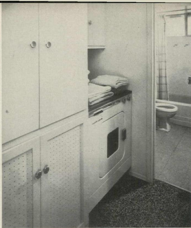
CORRIDOR LAUNDRY with combination washer-dryer, is used in models with the "B" bedroom wing (p 84). To save space, hot water tank is put on a platform, with clothes hamper built in under it.
