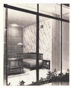
Folding wood doors, used as privacy screen above, come in heights to 12', widths to 18', or up to 15' x 50' for commercial use. Space-Saver doors come in choice of woods or finishes. Full length hinges are vinyl, glider suspension system is nylon.
