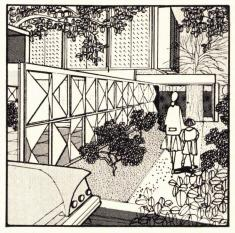
Here, the architect has conceived loadbearing walls of studs and aluminum panels, extended to enclose carport and patio . . . provide privacy, wind protection and a restricted space. Non-bearing part of the wall could be perforated or some panels omitted as the individual situation may require.
