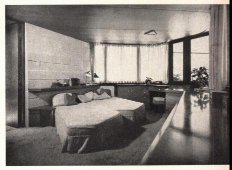
Bedroom also opens to a view of the garden. All walls are of standard 8"x8"x16" concrete block, set back ½" every second course. The result is a slight batter to the walls, and distinctive horizontal lines.
