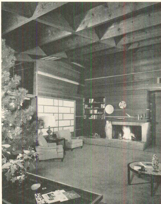
LIVING ROOM (right), like other rooms, has sloped ceiling. Low deck, at rear, extends over fireplace and cabinets. Translucent doors at left open to large balcony overlooking distant mountains. /END
