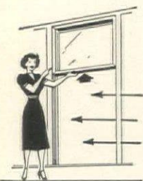
All panels at top—ventilation below head level.
