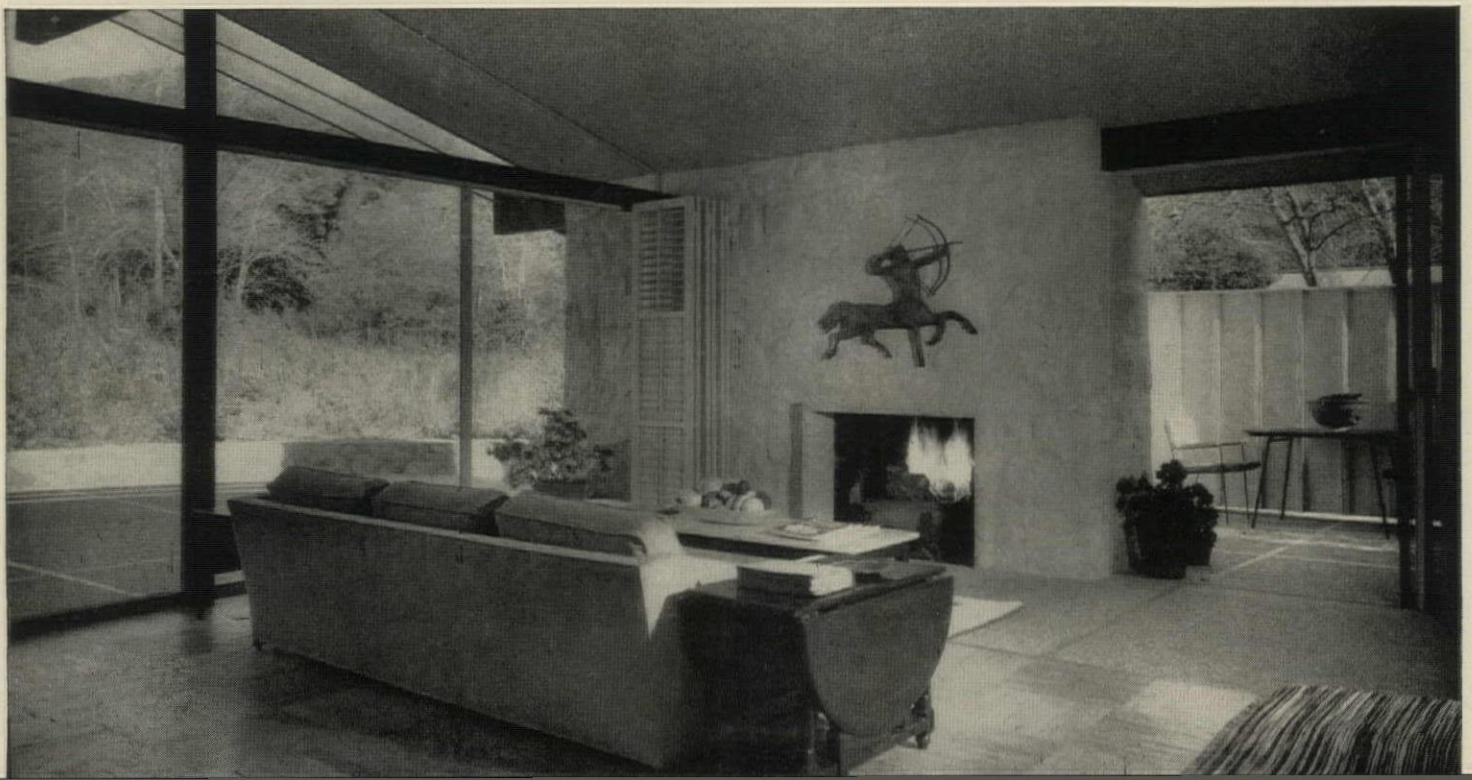
THE TEXTURED-PLASTER ceiling unites the indoors with the outdoors in the master suite living area ( Below ). Keymesh used over gypsum lath in this construction.
