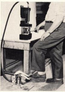
Hydraulic 5-ton vise is a high-speed fabricating tool for a wide variety of bending, shearing, punching, or holding jobs. Vise produces up to 10,000 psi. Jaws are 4½" wide, 3½" deep, open to 6". Pipe jaws hold up to 4" pipe; pipe bender will make 45° bends in 34" pipe; shear will cut 5%" stock.
