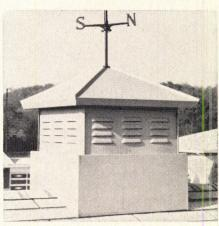
Steel cupola needs only to be nailed to the roof as it comes from carton, can be installed by one man in a few minutes. Extra flashing is needed if it is used as a vent housing. Several styles of weathervane are available as an optional extra. Basic unit is 30" square, 32" high (without vane), lists at \$39.75.
