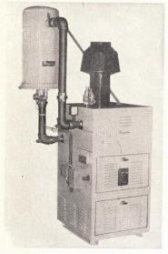
Swimming pool heater handles 30 to 40 gpm flow rate, produces temperature rise as low as 7F to 10F without condensation; recirculation system is said to prevent corrosion, scaling and electrolysis. "Lifelong" heater carries a 20-yr guar-
