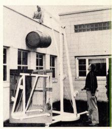
High-lift portable crane will lift 750-lb loads to 14'. Mast and brace telescope as a unit, are easily raised by mast-mounted hand winch. Maximum lift is 1,250 lb to 8'8". For outdoor use, crane has 10" wheels in front, 6" casters in rear.
