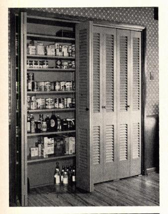
**Ideal bi-fold doors** have full-mortise hinges, can be used between rooms as well as on closets. Units are jamb-mounted. Top guide hangers and top and bottom pivot brackets are springloaded, self-squaring, and have self-lubricating nylon bushing. Units fit openings 6'8" high and 3', 4', 5', and 6' wide.
