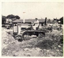
New bull-grader mounts on International T-340 crawler. Blade is 851/2" wide, can be set 1134" below grade, or raised 35" above ground. It can be angled from 25° right to 25° left. High lift capacity makes it work well on slopes, banks, and shoulders. Leverage is great enough to remove trees and stumps or cut ditches.
