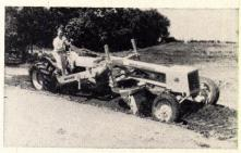
Low cost grader fits Massey-Ferguson model 202 industrial tractor. Lev-L-All will work as leveler, grader, maintainer. Standard equipment includes hydraulic leaning front wheels and lateral shift. Long wheelbase and short turning circle allows close maneuvering. Unit is easily attached or detached.
