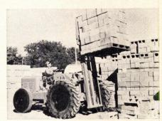
**6,000-lb fork lift** comes with standard 10' or optional 7' mast. Unit will work in rough terrain on-site or in a warehouse. Short wheelbase and oscillating rear axle give high maneuverability. Engine is 73 bhp, transmission is torque converter, steering is by power.
