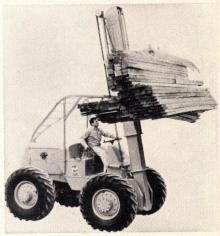
Hi-lifter fork truck has a new attachment: a combination lift arm and pallet fork. With it the hydraulic unit will lift a 2,000-lb palletized load up to 35'. Attachment will deliver brick, block, or stone to a third story.
