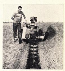
New 12-hp Ditch Witch will trenches to 12" wide, 5' deep. M-322 model is scaled up from popular M-3. New model will cut foundation footings, sewer laterals, drain fields, or bury utilities. Engine is an air-cooled 12-hp Wisconsin. Unit will dig 4" trench 5' deep, 12" trench 3' deep in any soil, maker claims.
