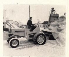
Reverse-mounted loader is designed for stock-pile work, has a self-loading 1-cu yd hydraulic bucket. Bucket is self-leveling. RL-400 mounts on utility tractors, has a lifting capacity of 3000 lbs, breakaway capacity of 4,500 lbs.
