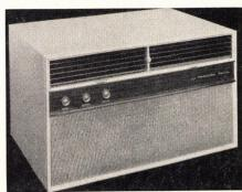
Frigidaire 1960 units offer "stereo" cooling: grille directs cooled air around room occupants, not at them. New pinfin coil speeds cooling and moisture removal. Polystyrene air guide cuts operating noise. Models come in 6,000 to 16,500 Btuh capacities.
