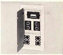
Fusible 100-amp entry has a single 100-amp Renu-Fuse to control all circuits, four 60-amp Renu-Fuses for range, dryer, air conditioner, workshop, etc, and up to 16 plug fuse circuits for lighting and appliance outlets. Device has a deadfront, comes in surface or flush mounting models. UL listed.
