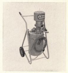
Aro airless spray atomizes paint by hydraulic pressure, provides heavier coats with less overspray. Pump works at 20:1 ratio to give 30 to 200 psi. Unit delivers 1/4 gpm at 20 cycles through two spray guns. Unit comes in 71/2-gal portable (illustrated) or 55-gal stationary models, with or without filters. Model shown is \$890 to industrial users.
