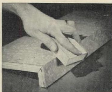
JOINT IS SO SHARP it may need slight sanding for safe handling.
