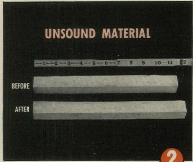
is sound—it has not expanded. Right: The two bars were made of one part portland cement and one part of a lime which does not meet autoclave test. Note expansion—proof of unsoundness.
