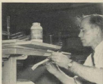
GLUE IS APPLIED freely to bevels. Waterproof glue is recommended.
