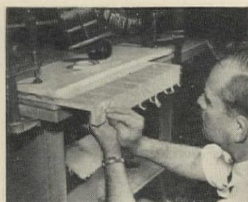
JOINT IS SO TRUE glued edge can be held in place by cellophane tape.
