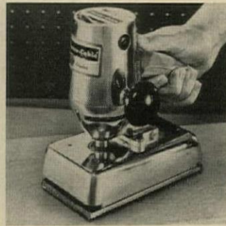
FINISH SANDER is standard size 5,000-rpm orbital unit.
