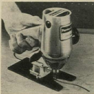
SCROLL SAW (23,000 rpm) cuts faster, smoother than sabre saw.
