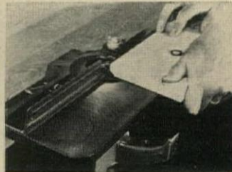
SHAPER TABLE cuts 3/4", jointer cuts 1 1/2"x3/32" deep.
