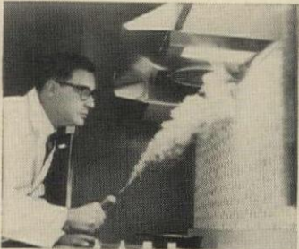
ODOR REMOVAL by range hood is checked visually with photo sequence showing smoke patterns.
