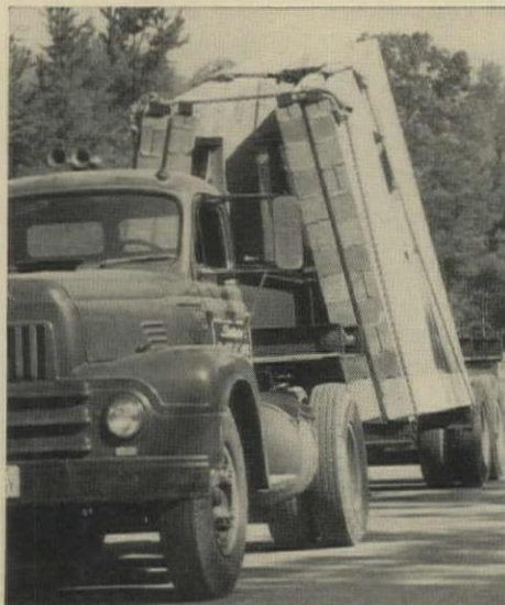
SPECIAL TRAILER carries finished wall panels, stacked like plate glass, from plant to site. Biggest panel weighs 3 tons and is 11'4" high.
