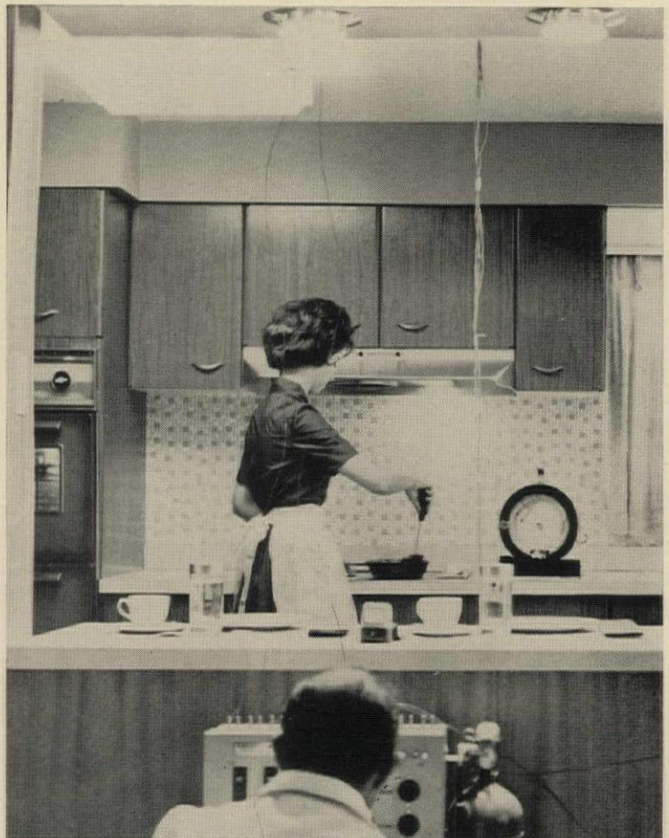
HEATING EFFECT of cooking and lighting is recorded, foreground, by use of thermocouples suspended over kitchen counter and range.
