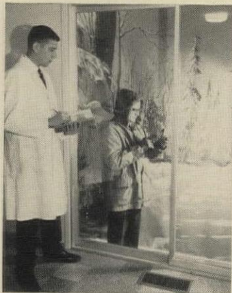
HEAT LOSS can be checked in summer by producing "winter weather" in lab's refrigerated room.
