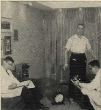
HEAT produced by electric system (plus lights) is checked on mannequin wired with thermocouples.
