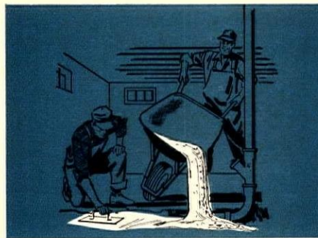
Cast iron soil pipe under the floor and to the street sewer gives maximum protection against infiltration, root penetration, crushing, pipe-joint failure. No substitute drainage piping can match it.
