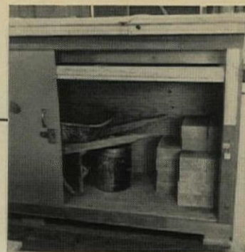
WHEELBARROW and pre-assembled corner blocks fit in compartment in rear of box.
