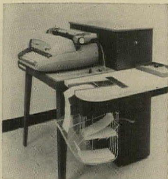
Automatic typewriter , fed by a card-sized folded tape, will type repetitive data at 100 words per minute. The unit also includes a device which punches the tape as the original is typed manually on the machine. Royal McBee, New York City.
