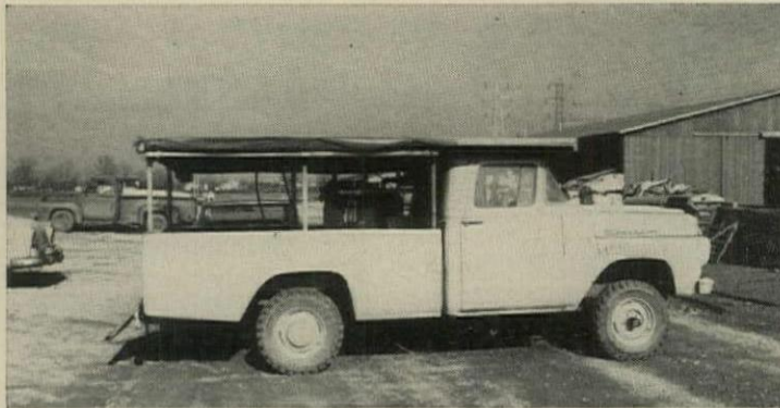
SPRAY-PAINTING TRUCK is equipped with a two-cylinder compressor powered by the truck's engine. A scaffold top above the body makes it easy for painters to reach high sections of the house.
