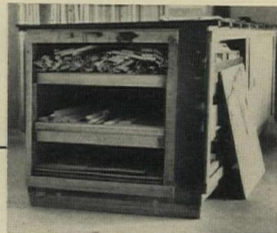
TRIM LUMBER is placed in full length shelves behind hardware storage. Sheet material is on bottom shelf.
