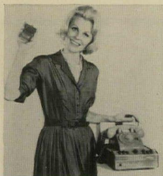
Electronic phone answerer records messages when phones are unattended, plays them back over the phone when given a code signal. The unit is portable, easy to install, and can be shifted from office to office. Phonomatic, Los Angeles.
