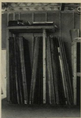
PREFINISHED PLYWOOD is stored vertically, sheathing, right, flat.
